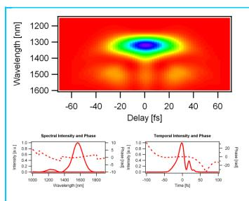
It shows a typical FROG trace. The pulse is from a fiber laser and the center wavelength is 1550nm. The pulse is suffering from a couple of chirp. After retrieving it, the program shows the temporal intensity and phase, and the spectral intensity and phase.
